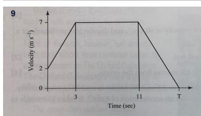
The diagram shows the velocity-time graph of the motion of a runner over a time period of *T* seconds. During that time, the runner travels a distance of 76 metres.
