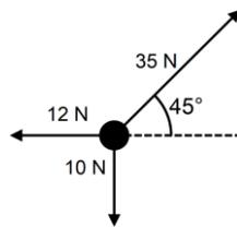
The forces shown in the diagram act on particle A of mass 0.8 kg. Calculate the magnitude of the acceleration of the particle
