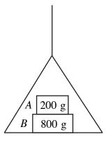
A light lift is attached to a vertical light inextensible string. The lift carries the masses A and B. The mass of A is 200 g and the mass of B is 800 g. Mass A rests on top of mass B as shown in the diagram above. The lift is raised vertically at 3 m s<sup>-2</sup>.
