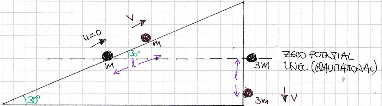
$$\underbrace{\cancel{KE_A} + \cancel{KE_B} + \cancel{PE_A} + \cancel{PE_B}}_{\text{ON RELEASE}} = \underbrace{KE_A + KE_B + PE_A + PE_B}_{\text{AFTER BOTH MASSES BY } l}$$
