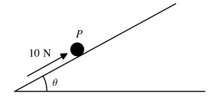
A particle P of mass 2 kg lies on a rough horizontal plane that is inclined at an angle  $\theta$  to the horizontal where  $\tan \theta = \frac{5}{12}$ . The particle is held at rest on the plane due to action of a force of magnitude 10 N which acts up the plane in a direction parallel to a line of greatest slope of the plane, as shown in the diagram. The particle is on the point of slipping up the plane.
