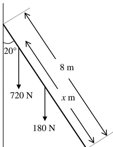
The system is in equilibrium with the ladder at  $20^\circ$  to the vertical.
