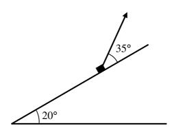
A box of mass 60 kg is held in limiting equilibrium, on a fixed rough inclined plane, by a rope. The plane is at an angle of 20° to the horizontal, as shown in the figure above.
