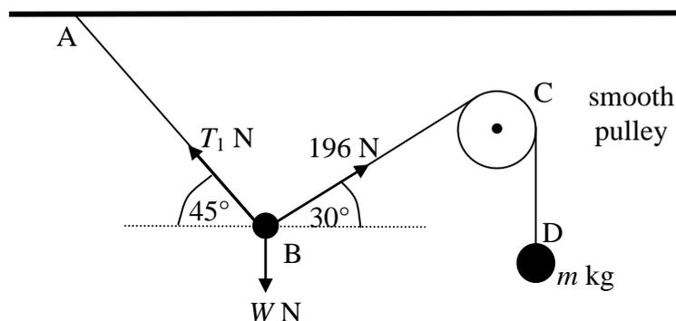
The diagram shows a load of weight  $W$  N at B in equilibrium. The load is attached by one light string to the ceiling at A and by a second light string that passes over a smooth pulley at C to an object of mass  $m$  kg hanging freely at D. The angles of the strings and the tensions  $T_1$  N and 196 N acting at B are shown in the diagram.
