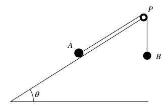
Two particles A and B, of equal mass are attached to each of the ends of a light inextensible string. The string passes over a smooth pulley P, at the top of a fixed rough plane, inclined at  $\theta$  to the horizontal, where  $\sin \theta = 0.28$ .
